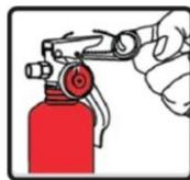
Set the extinguisher down. Hold it by the tank (pressure on the handle could pinch the pin). Pull the pin straight out.
